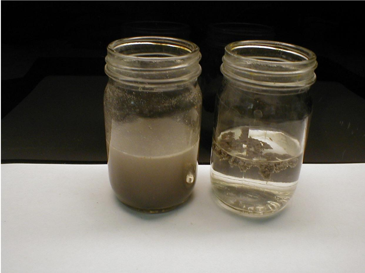
**Figure 3. Jar test of chocolate containing wastewater from Ricolino plant.**
