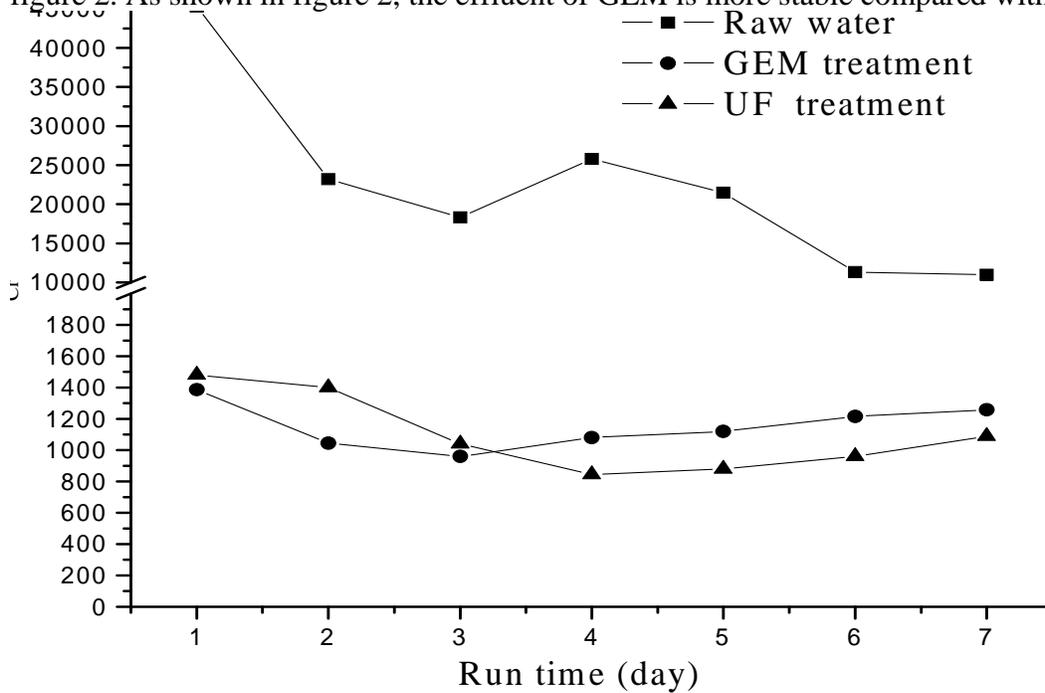
**Fig. 2 Effect of run time on the COD<sub>Cr</sub> of effluent**
