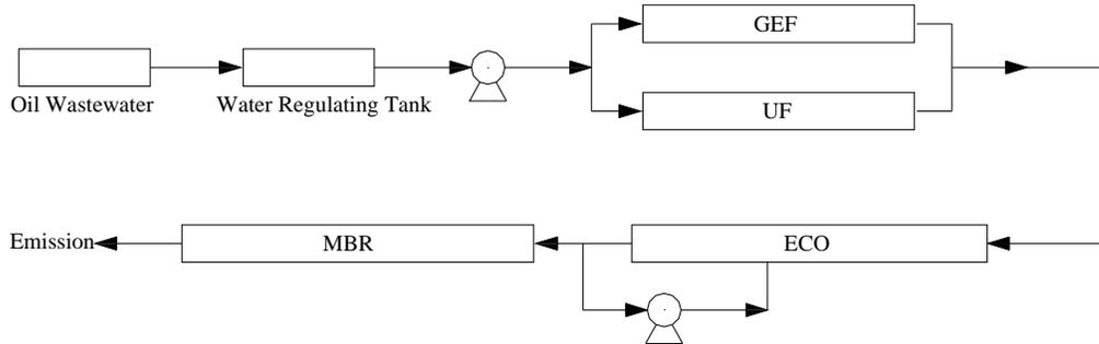
**Fig. 1** Flow chart of the effluent treatment processes.
