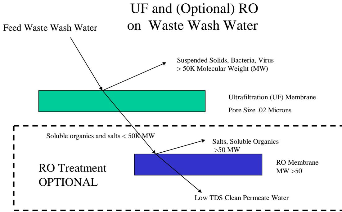
**Figure 2. UF-RO pilot system schematic**
