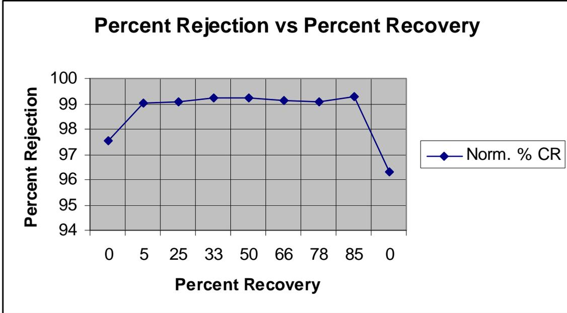
Figure 5. Percent rejection vs. Percent Recovery for RO membrane
