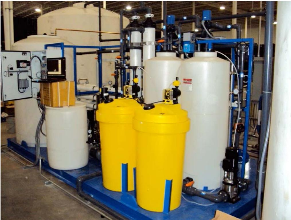
**Figure 7. Picture of the UF System**
