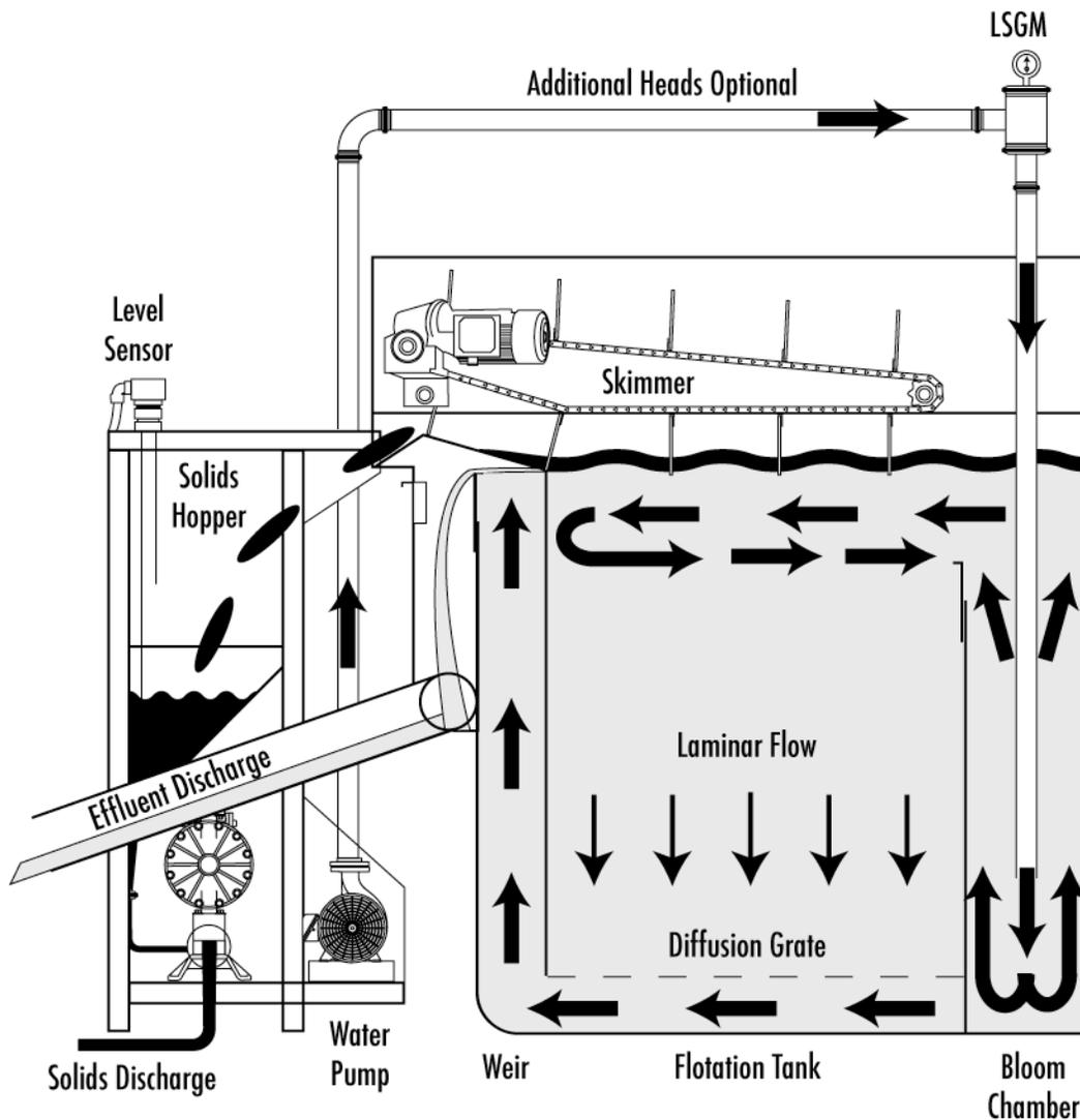
Coagulation, flocculation and flotation are among the most effective approaches to remove fats oils and grease, suspended solids and colloidal materials (even some proteins and
