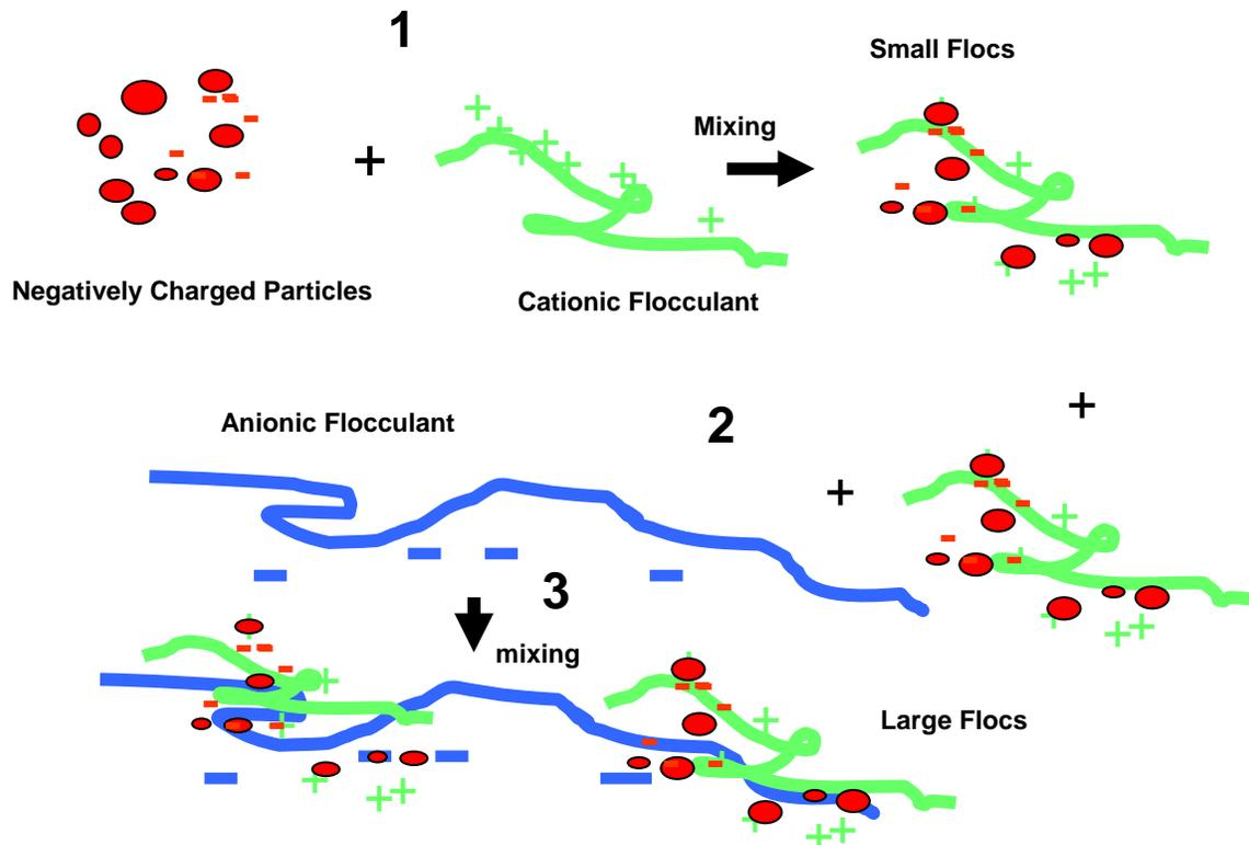
**Figure 4. Dual polymeric flocculant approach.**
