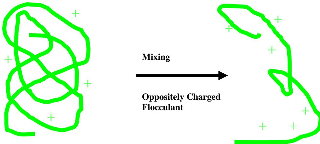
**Figure 6. Uncoiling of high molecular weight polymeric flocculant molecules.**
