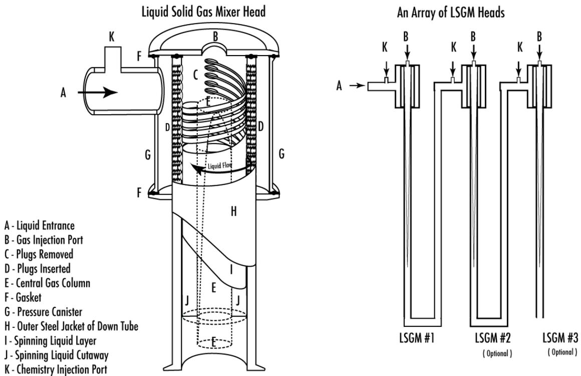
**Figure 2 – Schematic Presentation of the LCP/LSGM**
