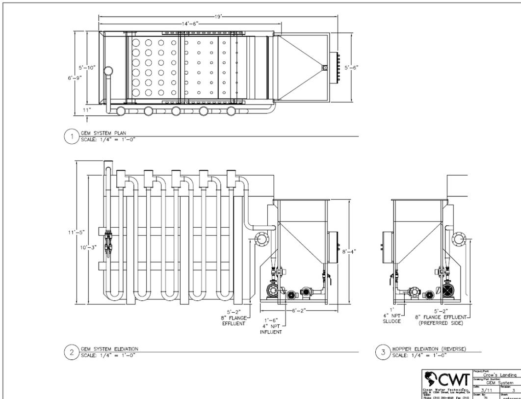
Figure 9. The Dimensions of the GEM System installed at the rendering plant
