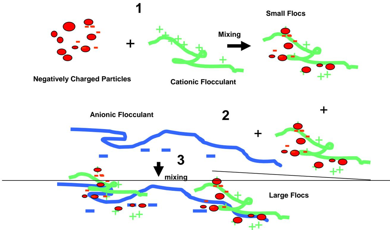
Figure 5. Dual polymeric flocculant approach.
