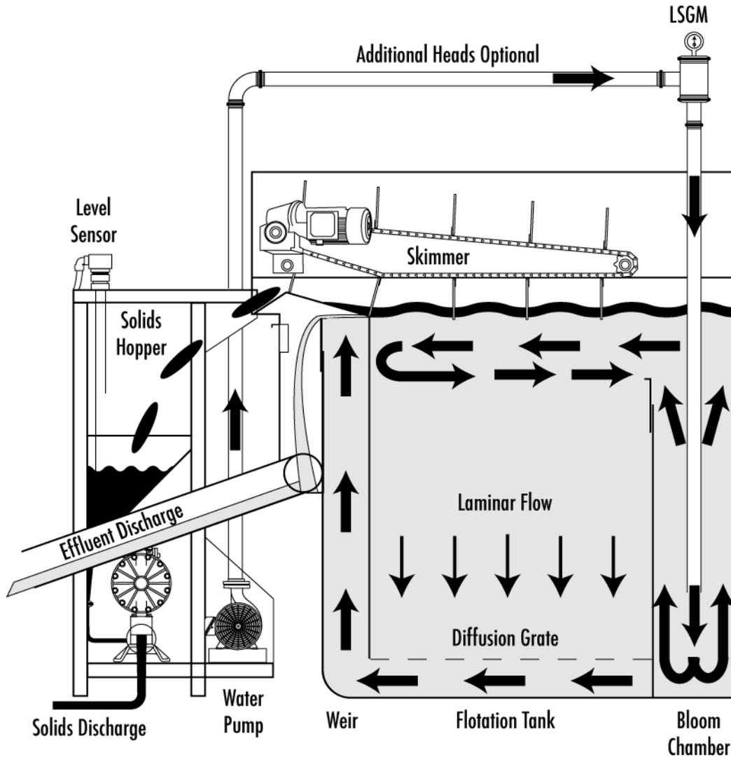
**Figure 4 – Schematic Presentation of the Hybrid Centrifugal – Dissolved Air Flotation System**
