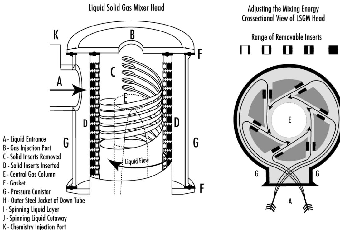
**Figure 3 – Schematic Presentation of the LSGM Heads**
