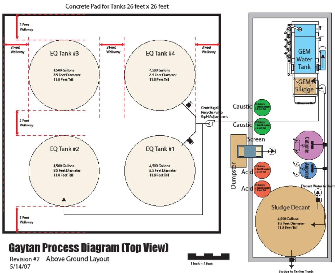
unpleasant odors (hydrogen sulfide). Pretreatment systems are often designed to remove maximum amount of TSS, FOG and macromolecules. Other dissolved contaminants can then be removed in the municipal treatment plants.
